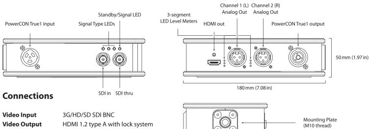
Video OutputHDMI 1.2 type A with lock system<br/>3G/HD/SD SDI BNC (reclocked loop thru)Audio Output2 x Balanced +4dB XLR (analog) with<br/>level meters
