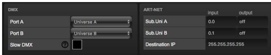
Figure 10.7: Converting Art-Net to DMX step 3
